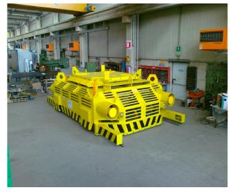
**C.M.P. SCRAP BUCKET CAR** is designed to charge scrap bucket avoiding typical damage suffered by traditional cars because of the scrap fall. Thanks to correctly designed outer shape, which is always "in the shadow" of the bucket, the scrap could be easily charged without worrying about its fall on the car and related damage and consequent loss of time and money.
