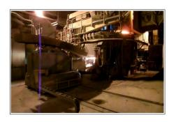
The adaptability and the simple and sturdy design of the **E.A.F. Scrap pusher and slag door cleaning robot complete with sampling manipulator,** allows every steel plant to be suitable for this application. In this way to operate, there is an average saving of 1-2 minutes every 50 minutes tap-to-tap time. This saved time represent an indispensable advantage to be implemented in every modern melt shop.
