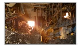
This cold scrap presence in the inner sill is prolonging the phase-on time to get the completed melted bath and the right metallurgical temperature. This extra time represents a dramatic increasing of the economic costs that cuts an important part of the final economic profit.
