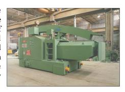
The engineering design of the **E.A.F. Scrap pusher and slag door cleaning robot complete with sampling manipulator** has been improving by the years and by feedbacks from our worldwide clients. The product has been constantly tested by the field and by complex numerical simulations of the physical reality. The action of the pushing arm is explicitly designed for reaching the sill cleaned from the scrap and the slag level control, in the safest and most durable way.
